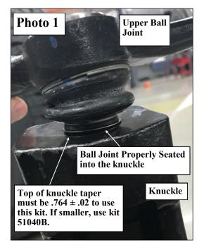
*IMPORTANT!: The inner CV* axle race can easily come out of the CV cup if the knuckle is pulled away from the vehicle. The knuckle should ALWAYS be kept vertical or pushed towards the center of the vehicle during the removal or installation of the upper control arm
