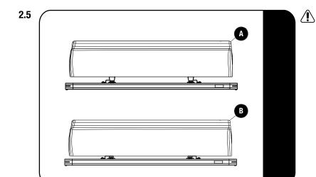
Hard shell tents may need additional support. If you are using these brackets with hard shell tents, such as James Baroud or Autohome, and you are unable to position the tent to rest directly on the rack side profiles (A), use TBMK009 – Hard Shell Tent Support Channels - by Front Runner (B) sold seperatly.
