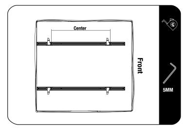
Measure the distance between the centers of Channel Feet to make sure it matches the position of the Rack Mount Brackets installed in Step 2.2.
