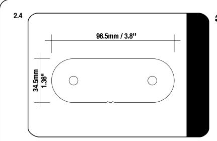
The Tent Channel Nut Plate included were designed for the Front Runner Tent but will also work with other popular tents. Check your mounting channel measurements for the appropriate size.
