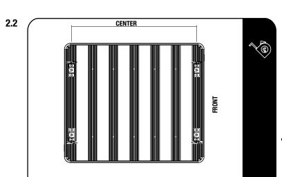
Measure the distance between the center points of the Rack Mount Brackets. You will need this measurement for fitting the Latch Bracket assembly to the tent channel in Step 2.6.
