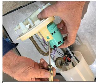
Photo 1: Remove OEM rollover valve
