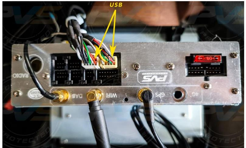
6. Feed other end of USB cables down to glove box for future access.
