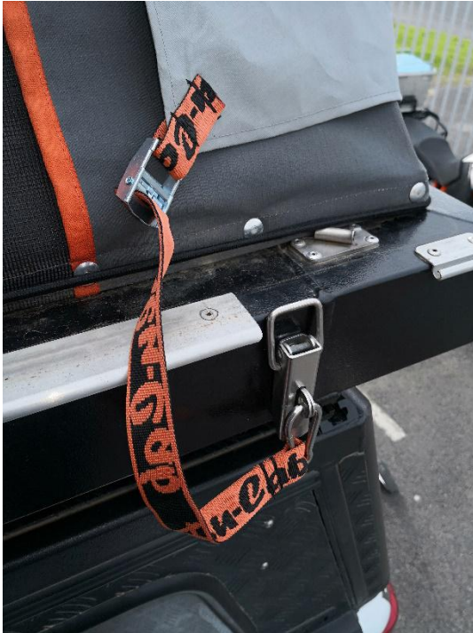
Spring hook attached to tent catch
