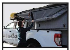
Step 7: When the third canvas fold is exposed, include it into the roll and carry on rolling upwards until the canvas roll is tight against the awning arms.
