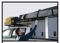
Step 3: Undo the three Velcro straps.
